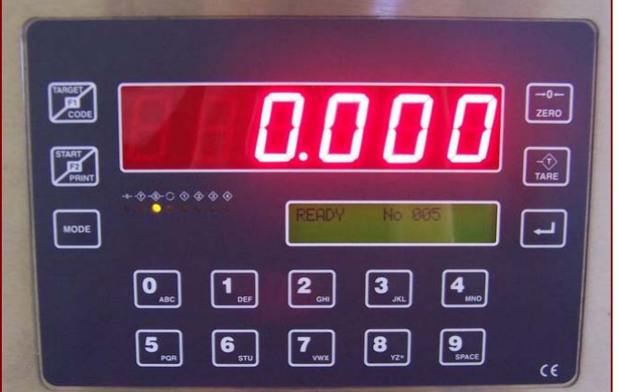
Optional LED display with 20 x 2 alphanumeric LCD
