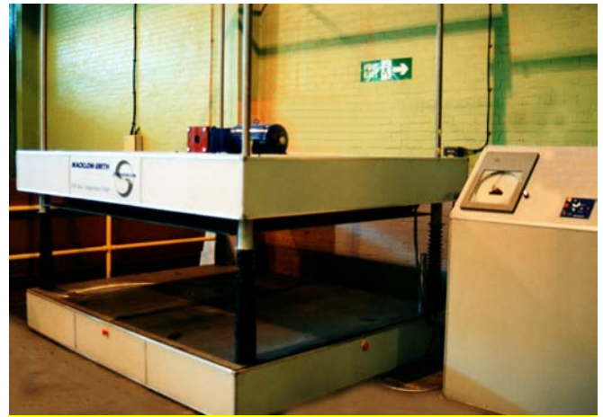
photo showing a large container tester during installation
